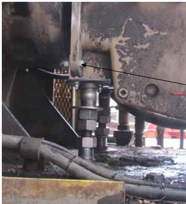
Left side through bolt
