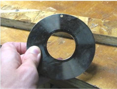
A 3 1/2" hard drive platter with the hole drilled through it.
