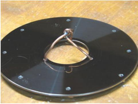
To support the chimes, make a hook assembly out of stiff copper wire. This assembly consists of one "U" shaped piece of wire and one (more or less) straight piece. The straight piece is soldered to the "U" shaped piece in the center. I wrapped the loose end of the straight piece back and down to keep it out of the way.
