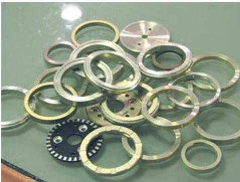
You'll also need various other junk from the hard drives. Pictured here are various findings from inside the hard drives. Most of these are spacer rings, used to space apart the platters on older hard drives. I used these as "beaters" in the wind chimes.
