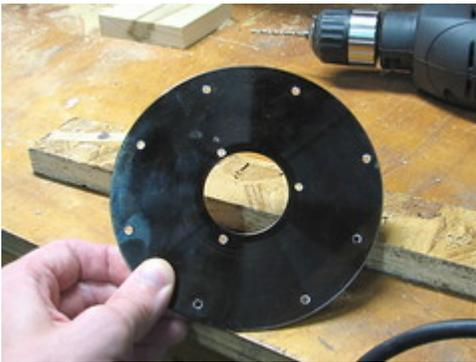
The top platter, 5 1/4", needs to have a hole around the edge for each dangling platter that it will support. Drill eight holes around the perimeter of the platter.
