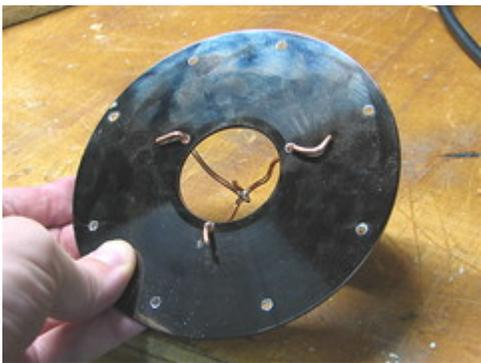
On the back side, the loose ends of the copper hook assembly are folded back to keep the hook anchored in place.
